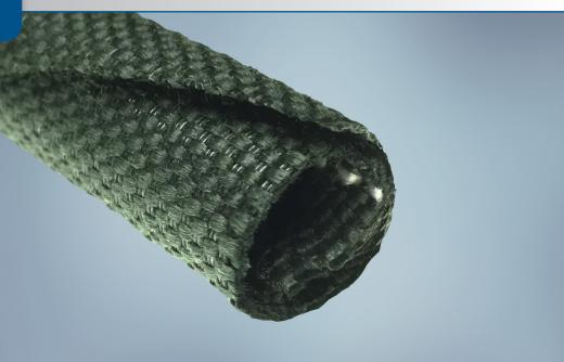
**TwistTube® 2440** is a high temperature, lightweight sleeve designed to provide a combination of thermal and mechanical protection. It incorporates a unique self-wrapping closure that allows for quick and easy installation. It also allows for breakouts and can be installed over completed assemblies. The overwrapping design of the product allows it to maintain a circular profile when flexed.
