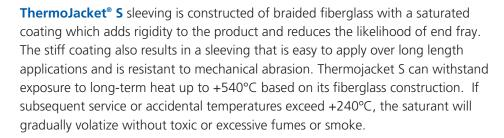
ThermoJacket sleeving provides excellent long-term heat protection for hoses, wire harnesses and cables. ThermoJacket is available in a variety of grades, offering industrial users the option of selecting combination of properties best suited to their specific application.
