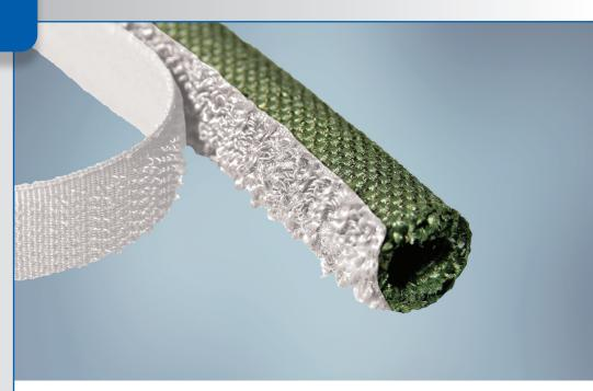
**ROUNDIT® 2000 NX GRIP** is a woven combination of Nomex® and PPS (polyphenylene sulfide). The Nomex/PPS blend in a flat weave construction gives ROUNDIT 2000 NX GRIP a rugged yet smooth texture and appearance for high temperature bundling and abrasion resistance. This product is rated to +200°C (+392°F) and is non-halogenated.
