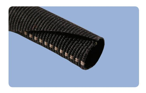
**ROUNDIT® 2000 LX** is a self-wrapping sleeve used for abrasion protection of wire and cable bundles. It is woven from a blend of PPS (polyphenylene sulfide) multifilaments with an oil and water repellant treatment. The wrappable construction was designed in order to minimize weight while maintaining 100% coverage, resulting in an optimized combination of lightweight materials and abrasion resistance.
