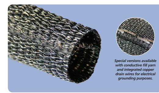
**ROUNDIT® 2000 Cu EMI** is a self-wrapping sleeve designed to provide >40dB of electromagnetic (EM) screening attenuation. Tinned copper wire is combined with polyester yarn to create a wrappable product that offers flexibility and consistent shielding protection. The product features an acrylic/silicone coating to prevent end fray and enable cold cutting for specific product lengths.
