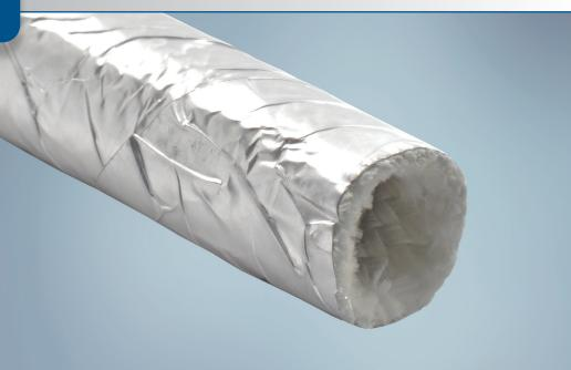
**ReflectSleeve® 1400** is a flexible, aluminized, high bulk, fiberglass sleeve used to protect components in high temperature environments. ReflectSleeve 1400 features an outer layer of spiral wrapped aluminum foil that reflects radiant heat while providing a barrier against moisture and other damaging elements. The inner layer of high bulk fiberglass has natural air pockets which greatly increase insulating efficiency.
