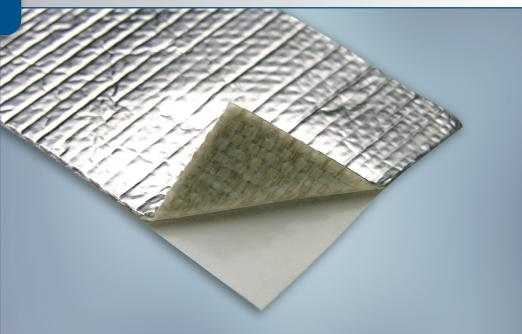
**ReflectShield® 1805** is a woven fiberglass fabric that has an aluminum foil laminated to its outer surface and a pressure sensitive adhesive on its inner surface. The unique, multipolymer adhesive exhibits high adhesion to low surface energy plastics such as HDPE, polypropylene and gas filled polypropylene. It has been designed to show very good adhesion properties also after heat ageing and fluid projections.
