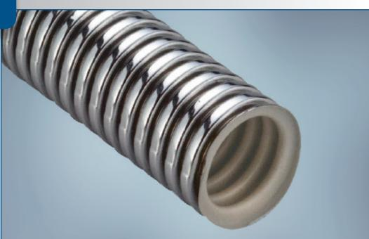
**ReflecTube® 1597J** is a reflective convolute tube designed to provide thermal protection for components in radiant heat environments. Composed of a modified nylon polymer base substrate and a highly reflective aluminum coating, ReflecTube 1597J provides protection for wires, cables, hoses and other components requiring radiant heat protection in close proximity to engine and exhaust systems.
