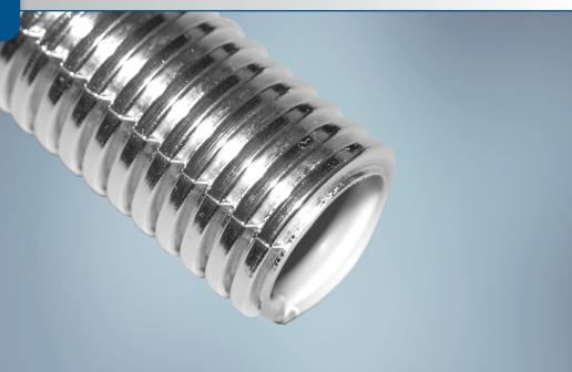
**ReflecTube® 1592** is a reflective convolute sleeve designed to provide thermal protection for components in radiant heat environments. Composed of a high temperature nylon 4,6 polymer base substrate and a highly reflective coating, ReflecTube 1592 provides protection for wires, cables and hoses in applications that have radiant heat source temperatures as high as +538°C (+1000°F).
