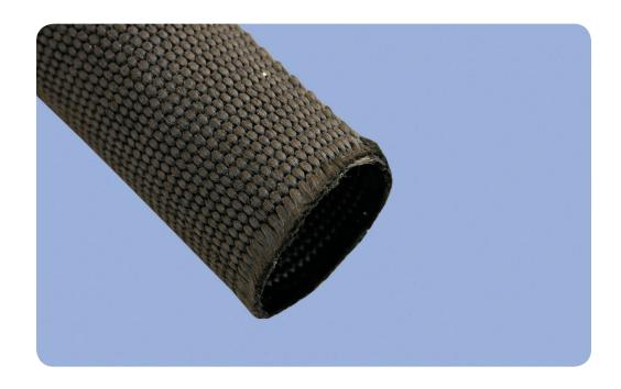
**ProGard®** is a durable, woven nylon sleeve constructed of high denier nylon yarn. ProGard provides enhanced abrasion protection over hose assemblies, cables, wires and other applications where rugged environments may cause wires and hoses to be chafed and damaged.
