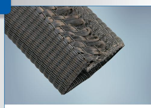
**Hookit<sup>™</sup>** is a lightweight, damage-resistant sleeving used to protect and dress wiring and hose assemblies. Its patented hook and integral loop closing feature eliminates the need for an open end for installation. Hookit oversleeve permits quick and easy access for inspection, rework or replacement of components.
