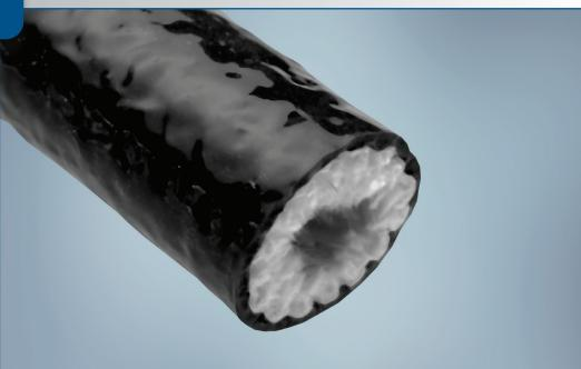
**FyreJacket® 1610** is a thickwall braided fiberglass sleeve coated with silicone rubber that provides thermal protection. FyreJacket 1610 is used to protect hoses, lines and cables in high temperature areas. It additionally provides protection against short-term hazards such as flame blasts. When burn-through is a threat, the specially designed sleeve construction retards the penetration of the flame. This can allow critical components to continue to function for a short amount of time.
