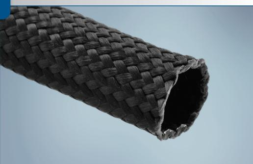
**FlexFit® 2118** is a flexible, slightly expandable sleeve specifically designed for abrasion/ mechanical protection of wire harnesses, tubing and hoses. Braided with polyester multifilaments, it is lightweight, and rugged yet has a very attractive appearance. A high coverage ratio contributes to the product's aesthetic appeal and makes it suitable for visible applications.
