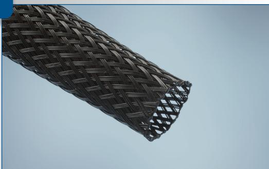
**FlexFit® 2112** is an expandable sleeving specifically designed for the abrasion protection of automotive wire harnesses, cables, tubings and hoses. Its specific structure combines both a high coverage ratio and a high expansion ratio which enables installation over long lengths even after the fitting of end connectors. It also allows a large number of diameters to be covered with a limited range of sizes.
