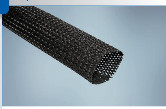
**Expando® PT & Expando® PT Plus** are tough, lightweight oversleeves used to protect cable assemblies, hoses and wire harnesses from chafing, cutting and abrading. The open-braid construction of Expando products enables each size to expand to fit several application shapes and diameters. This open-textile construction also makes them highly flexible and resistant to trapping water, heat and humidity.
