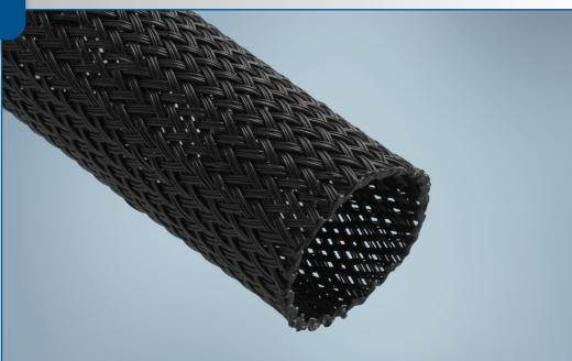
**Expando® DM TW** is a lightweight and flexible braided sleeve designed to provide mechanical protection for most common automotive applications. Constructed of PA (polyamide) monofilament guard strands and PET (polyethylene terephthalate) support strands, this dual-monofilament blend provides an excellent balance of abrasion protection, temperature resistance, and installability.
