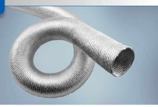
**Clevaflex® AFS-F-AFS** is a reflective corrugated tube designed to provide thermal protection for components in radiant heat environments. Its multi-ply construction of aluminum laminated fiberglass coupled with aluminum fiberglass scrim interior and exterior layers allows for good insulation to components requiring stable temperatures for optimum performance efficiency.
